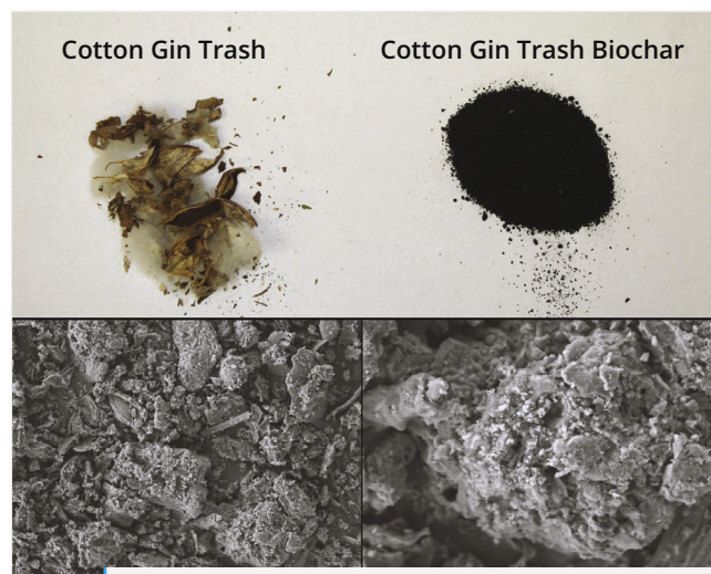
Figure 6. Cotton gin trash: Gin trash is a mix of burs (material that surrounds the boll), stems, leaves, seeds, and unrecovered lint. It contains a mixture of structured and less structured materials that result in a mixed biochar with respect to porosity. Seeds and woody bracts preserve some of their structure. This gin trash biochar shows evidence of salt crystallization (bottom right, 2,500x magnification).
