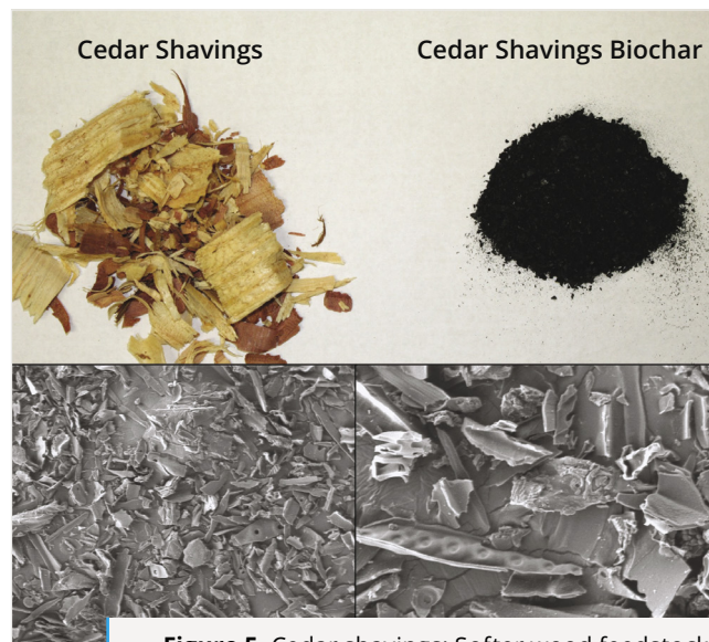
Figure 5. Cedar shavings: Softer wood feedstocks are intermediate in structure preservation between paper and hardwood. Starting with thinner shavings means less is preserved than with the mesquite.
