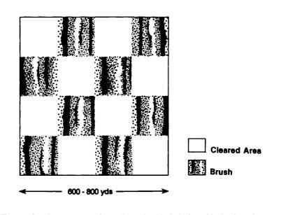
Figure 1. Brush management in an alternating block design with clearings that are 150-200 yards wide.
