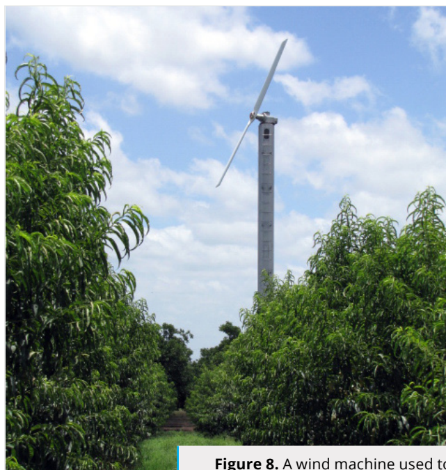
Figure 8. A wind machine used to protect crops during radiative frosts.
