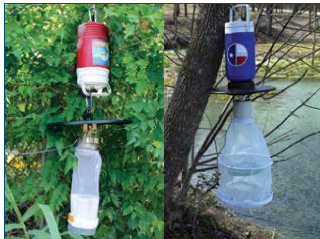
Figure 38. CDC light traps, each baited with a cooler of dry ice that releases carbon dioxide to attract female mosquitoes. Image sources: Gabriel Hamer and Mike Merchant
