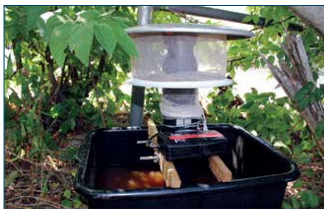
Figure 37. A gravid trap collecting gravid Cx. quinquefasciatus females. Image source: Gabriel Hamer
